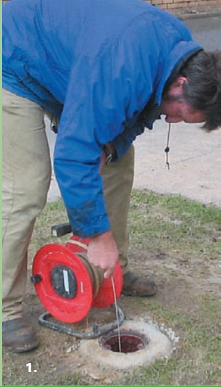
1. Measuring standing water level (Colac, Victoria); 2. Completed piezometer at a mine site (Ardlethan, NSW); 3. Hollow augering through a clay aquitard (Horsham, Victoria).
