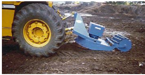
The Rotocult is made in Australia and is used to mix soil as thoroughly as a pug mill for much less cost and at a greater through-put.
